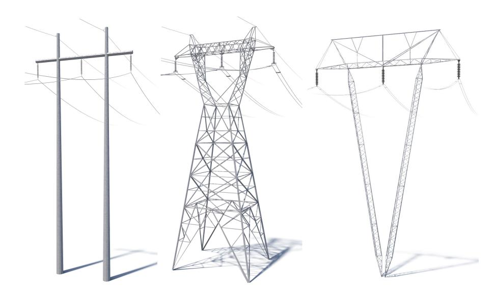
Crews plan to rebuild the line using primarily guyed-V, H-frames and lattice towers.
